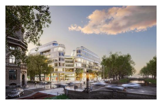
More than 40 percent of the development consists of the adaptive re-use and re-cladding of the original structure, significantly reducing the project's embodied carbon. Key historic elements – including the monumental stone façade from the 1907 Commerzbank building – have been thoughtfully preserved and reintegrated. The project has already been awarded a DGNB Platinum pre-certificate and Smartscore certification, contributing to its advanced sustainability profile.
